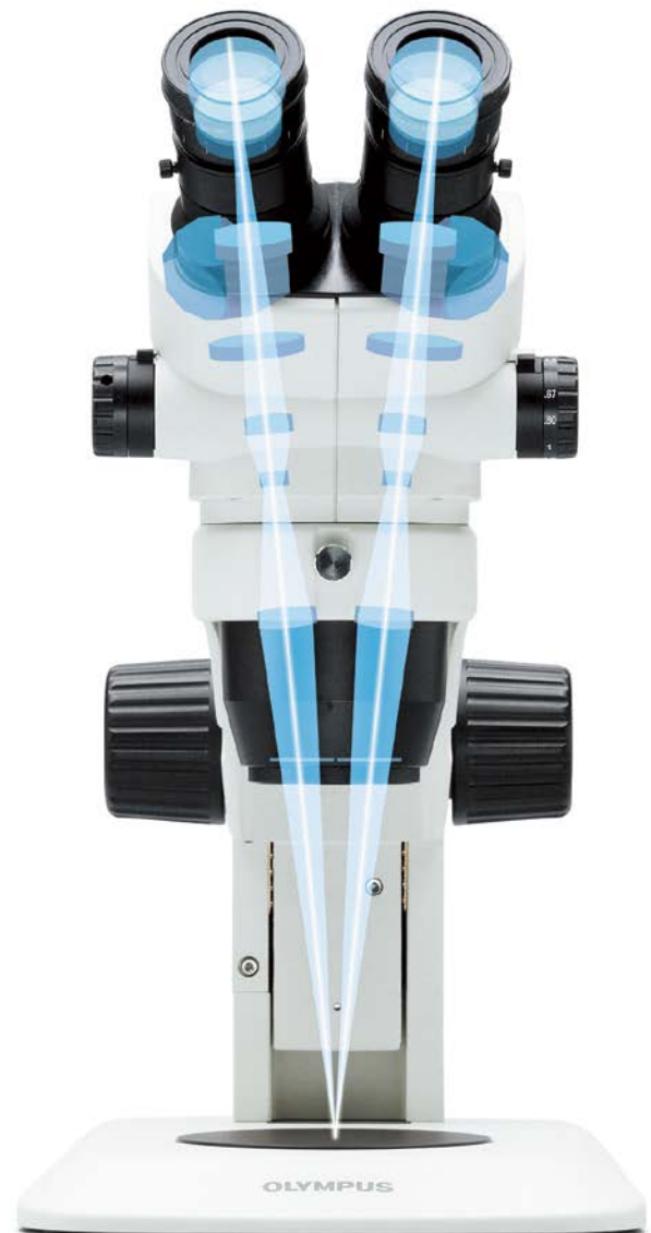
The Greenough optical system has two zoom optical paths inclined at a 10° angle. This enables a compact microscope design with high performance.
