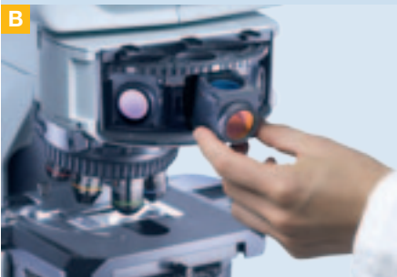
Easy replacement of filter cubes
