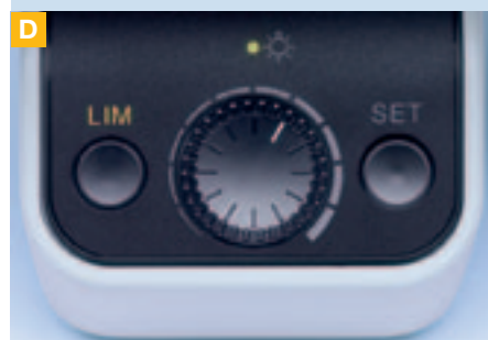
Integrated light intensity management on BX43
